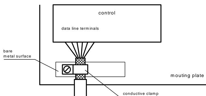
The cable shielding is to be connected at both cable ends. If equipotential bonding currents are expected due to the cable arrangement, electrical isolation is to be performed on one side. In this case, capacitive connection (approx.  $0.1\mu\text{F}/600\text{ V AC}$ ) of the shielding on the isolated side must occur.
