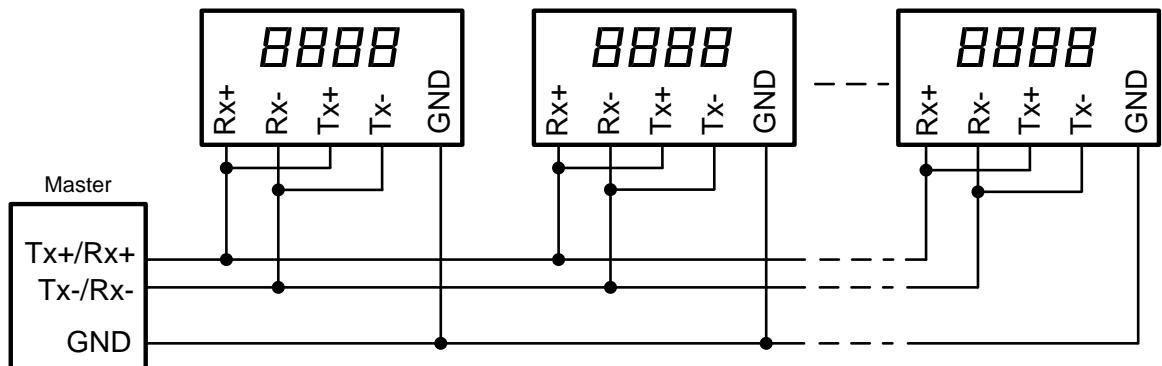
As an option interfacing can be effected via a RS485 4-wire bus (optional four-wire Modbus definition) as described as follows.
